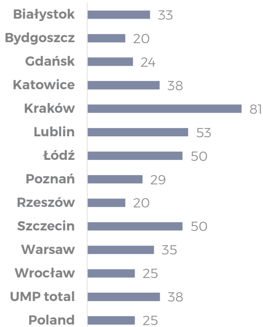
Number of water supply network failures per 100 km of the network in UMP cities in 2021
